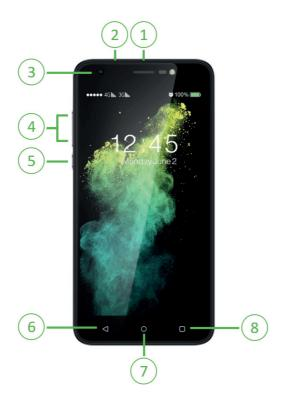
**Charging socket** (no. 1 in the picture below) is used for connecting the USB charging cable. By connecting your phone to a computer, you may take advantage of other available functions (see section Connecting to a computer).
