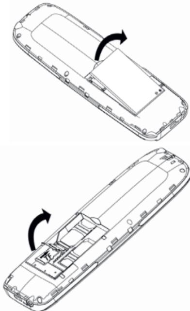
**Insert the SIM cards** in the appropriate slots under the battery with contacts facing down so that the SIM cards contacts touch the integrated phone SIM contacts. Insert SIM 1 card into the bottom right slot with the bevelled corner located in the top left corner of the slot, and insert SIM 2 card into the top left SIM slot with the bevelled corner located in the bottom right corner of the slot.
