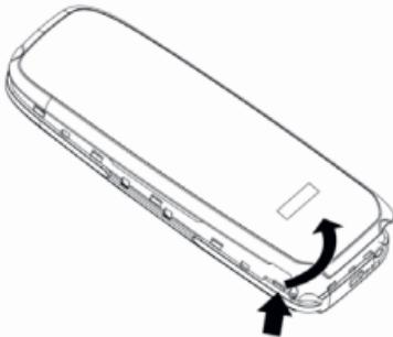
Lift the battery with your fingernail or a blunt object on top of the battery.
