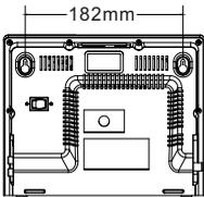
Fix the two nails (Size:3.5\*25BA) into the wall and they should parallel each other. (The distance between the two nails should be 182mm)
