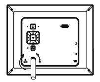
Attaching the stand: rotate the stand clockwise until it is fixed tightly in position.
