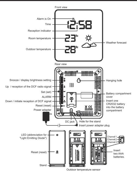
The device consists of the main unit with a radio-controlled clock and one outdoor temperature measuring unit equipped with a temperature sensor. The measured temperature is wirelessly transmitted to the main unit and displayed on its display. It is possible connect only one temperature measuring unit.
