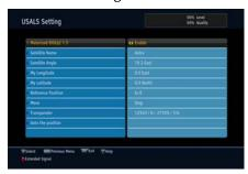
USALS (Universal Satellite Automatic Location System), also known as DiSEqC 1.3, will calculate positions of visible satellites just by pointing it to a known satellites.
