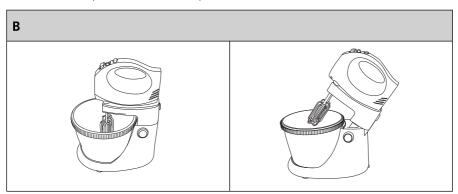
Press button (a) to release the lock of the motor unit (b) and with the other hand remove the motor unit (c). To release the attachments press button (a) and remove the attachments.
