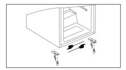
Unscrew the top pin and screw it in on the opposite side. Attach the door into the top pin and close it. Using bolts to screw in the pin of the holder on the other side of the appliance.
