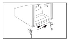
Unscrew the top pin and screw it in on the opposite side. Attach the door into the top pin and close it. Using bolts to screw in the pin of the holder on the other side of the appliance.
