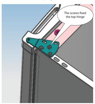
3 Replace the top-hinge and the door limit block and the door bearing bush to the other side A replace the top-hinge.
