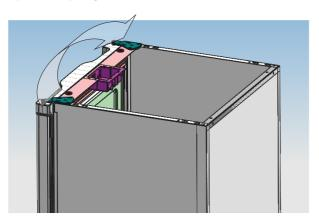
B replace the door bearing bush and the limit block.
