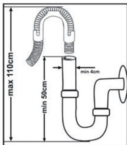
Connect the water drain hose directly to water drain hole or to the sink outlet spigot. This connection should be minimum 50 cm and maximum 110 cm from floor plane.
