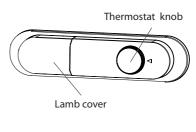
The fridge freezer thermostat automatically regulates the inside temperature of the compartments. By rotating the knob from position 1 to 5, colder temperatures can be obtained.
