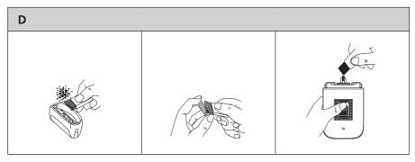
After cleaning, properly put the swivel unit with the shaving blades A<sup>(4)</sup> back in its place. Put the foil A<sup>(2)</sup> back into the cover A<sup>(3)</sup> while ensuring that the hooks on the inner side of the cover A<sup>(3)</sup> slide into the holes on the sides of the foil A<sup>(2)</sup>. Place the cover A<sup>(3)</sup> on to the shaving blade unit A<sup>(4)</sup>. Finally, do not forget to put on the shaving foil protective cover A<sup>(3)</sup>.
