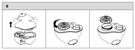
3. Fill the water tank A② with clean cold tap water. After filling up the water tank A②, properly screw in the plug A③ clockwise. Turn the water tank A② upside down with the plug A③ facing downwards and place it back on to the base unit A⑪ so that both parts fit into each other properly. When the water tank A② is placed on the base unit A⑪, water will start flowing into the water holder A⑨.
