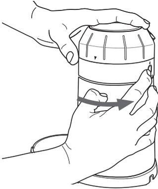
3. Press and hold the UNLOCK button at the back of the grinder base. Turn the milling fineness control knob anticlockwise with your other hand until the graphic mark on the milling fineness control is aligned with the one on the grinder base. This upper millstone can be only removed in this way - see figure below.
