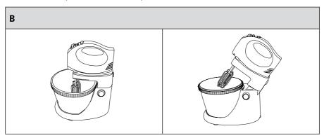
Press button ③ to release the lock of the motor unit ⑦ and with the other hand remove the motor unit ⑦. To release the attachments press button ③ and remove the attachments.
