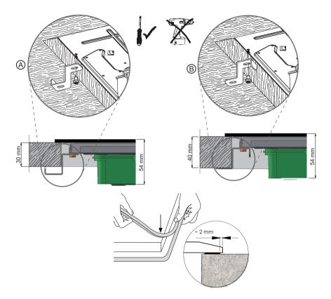
Insert the cooktop into the cut-out hole in the workbench.
