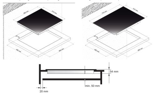
Cut out an opening of the corresponding dimensions according to the picture here provided.
