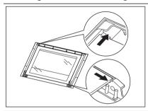
When the cleaning is completed, install the glass panel and the oven door. Do the above steps in the opposite sequence. The screen-printing zone must face the inner side of the door. Make sure that after the installation the surface of the glass panel frame on the screen-printing zones is not rough when you touch it.
