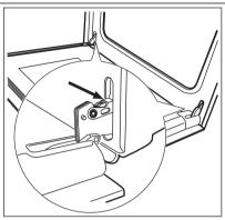
Open the door fully and hold the two door hinges.
