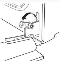
2. Lift and turn the levers on the two hing-
