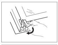
**5.** Release the locking system to remove the internal glass panel.
