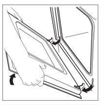
**3.** Close the oven door to the first opening position (halfway). Then pull forward and remove the door from its seat.
