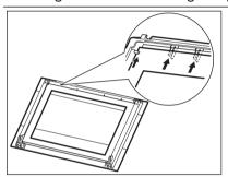
When the cleaning is completed, install the glass panels and the oven door. Do the above steps in the opposite sequence. Make sure that you put the glass panels back in the correct sequence. The middle panel has a decorative frame. The screen-printing zone must face the inner side of the door. Make sure that after the installation the surface of the glass panel frame on the screen-printing zones is not rough when you touch it.
