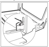
1. Open the door fully and hold the two door hinges.
