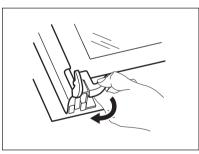
**5.** Release the locking system to remove the glass panels.
