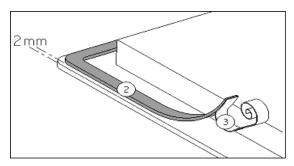
Insert the cooktop into the cut-out hole in the workbench.
