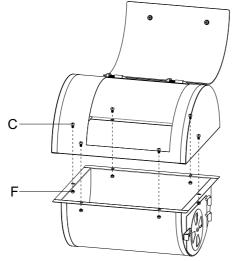
Please install and fix the ONE SIDE (Front) two holes to match the lid and fire bowl , then adjust the OTHER SIDE(Back) of the up and down hole position
