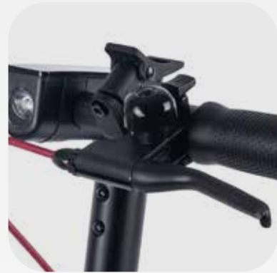
SAFETY Reliable rear disc brake and bell for audible signaling.
