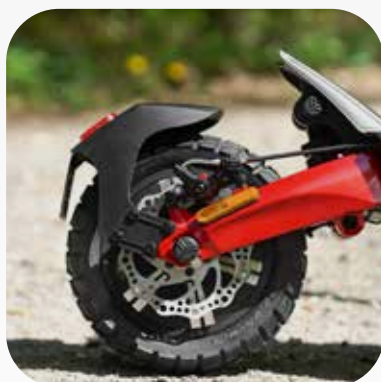
RELIABLE BRAKES Dual braking system - electric motor and mechanical disc brakes.
